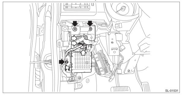
4) Remove IG relay 1 (push button start) (A) from the relay holder.
